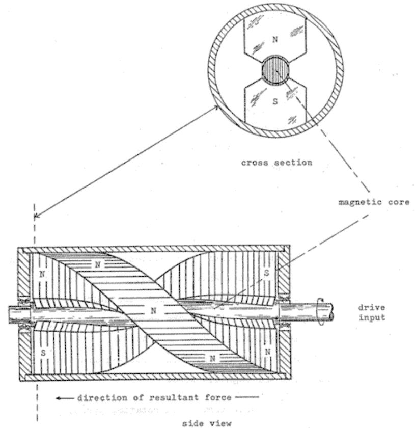
Figure 4. Linear Force Machine (magnetic)
