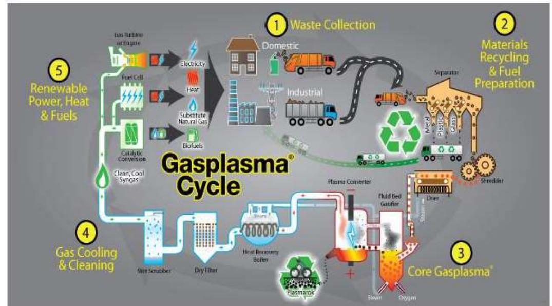
Advanced Plasma Power's advanced Gasplasma® technology today delivers 50% electrical conversion efficiency – twice that of conventional steam cycle technologies.
