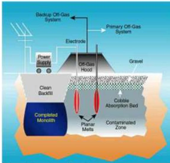
Planar melting system schematic.
