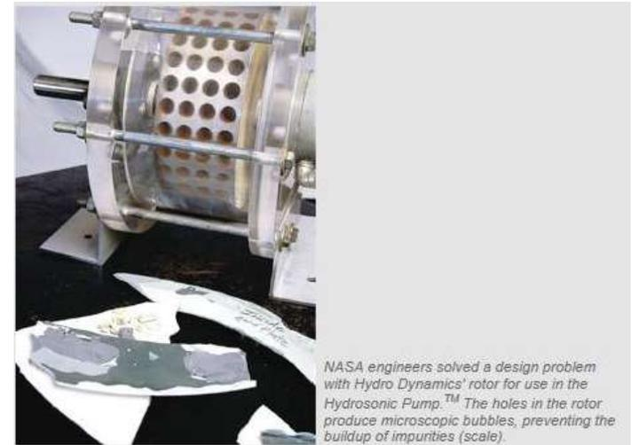
*NASA engineers solved a design problem with Hydro Dynamics' rotor for use in the Hydrosonic Pump™. The holes in the rotor produce microscopic bubbles, preventing the buildup of impurities (scale).*
