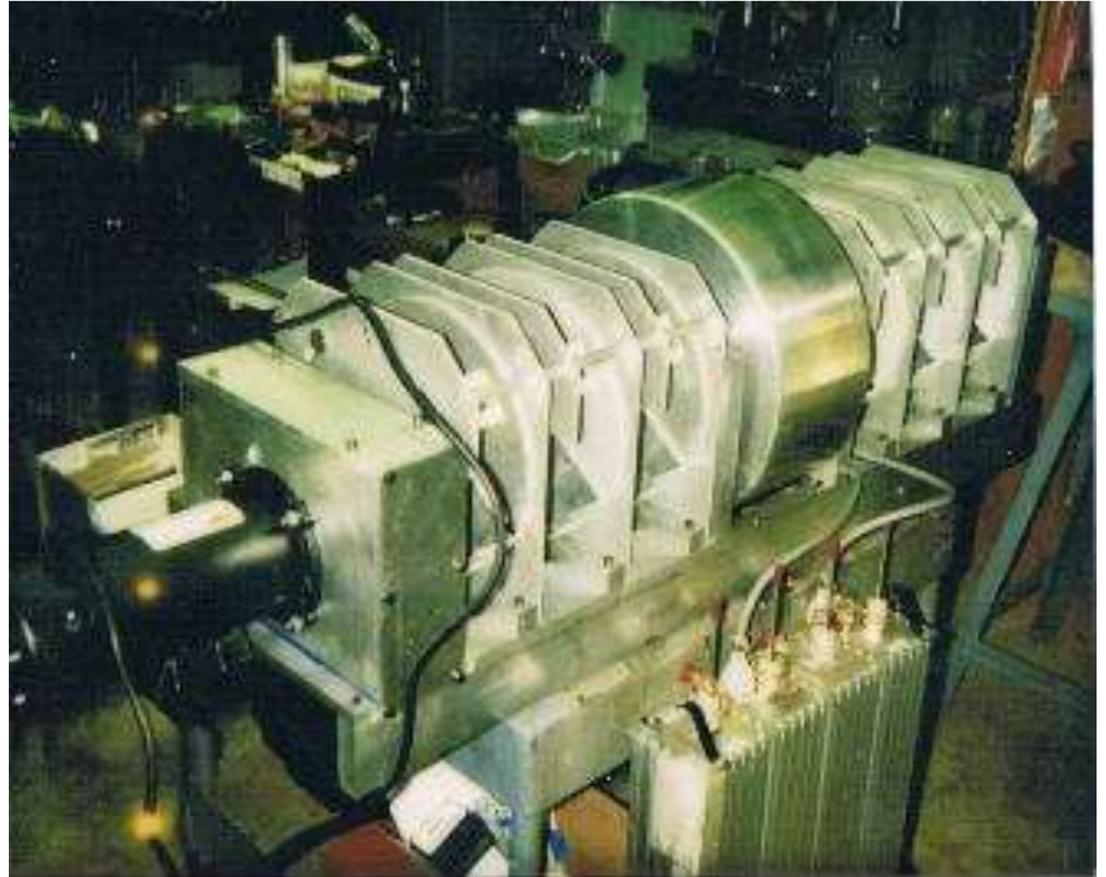
homopolar motor-generator. It was estimated that the cost of such an advanced electrical generator to be approximately the cost of installing smoke scrubbers on one coal-fired generating unit.
